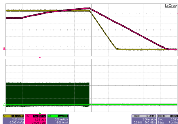
Figure 32 – Standby OV Protection.
