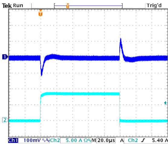
Load Transient: V_{IN} = 6.2V , V_{OUT} = 1.5V Ch.1: V_{OUT} , Ch.2: I_{LOAD} 0↔8A (slew rate \geq 10A/\mu S ) C_{IN} \approx 2 \times 47\mu F , C_{OUT} \approx 2 \times 47\mu F
