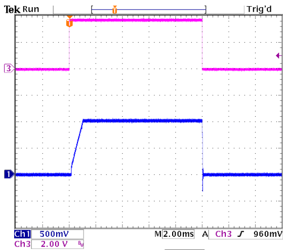
Power Up/Down at 8A (0.08 Ω) Load: V_{IN}/V_{OUT} = 5.0V/1.0V , 15nF soft-start capacitor, Ch.3: ENABLE, Ch.1: V_{OUT}
