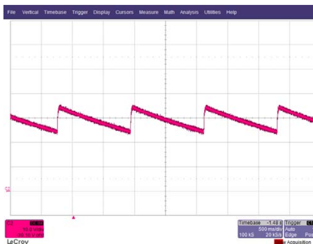
Figure 28 – Output Voltage: 230 VAC. V_{\text{OUT}} , 10 V / div., 500 ms / div.
