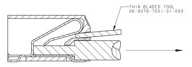
PUSH BLADE (NOT SHARP) INTO SLOT ABOVE WIRE. WHEN WIRE IS FREE, PULL TO EXTRACT.
