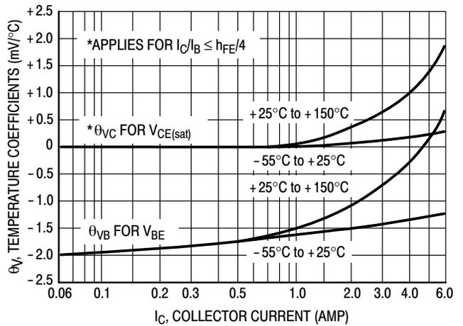
Figure 11. Temperature Coefficients
