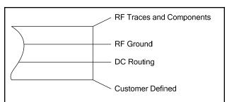
The PCB dielectric between RF traces and RF ground layers should be chosen to reduce RF discontinuities between 50  $\Omega$ M/A-COM recommends an lines and package pins. FR-4 dielectric thickness of 0.008" (0.2 mm) yielding a 50  $\Omega$ line width of 0.015" (0.38). The recommended metalization is 1 ounce copper.
