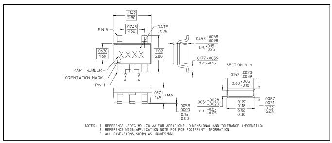
Reference Application Note M538 for lead-free solder reflow recommendations. Meets JEDEC moisture sensitivity level 1 requirements.
