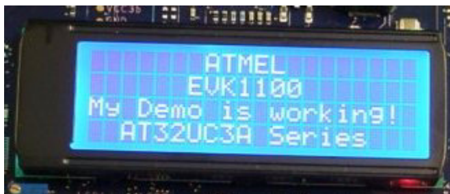
Figure 6-50. LCD Display showing edited message
