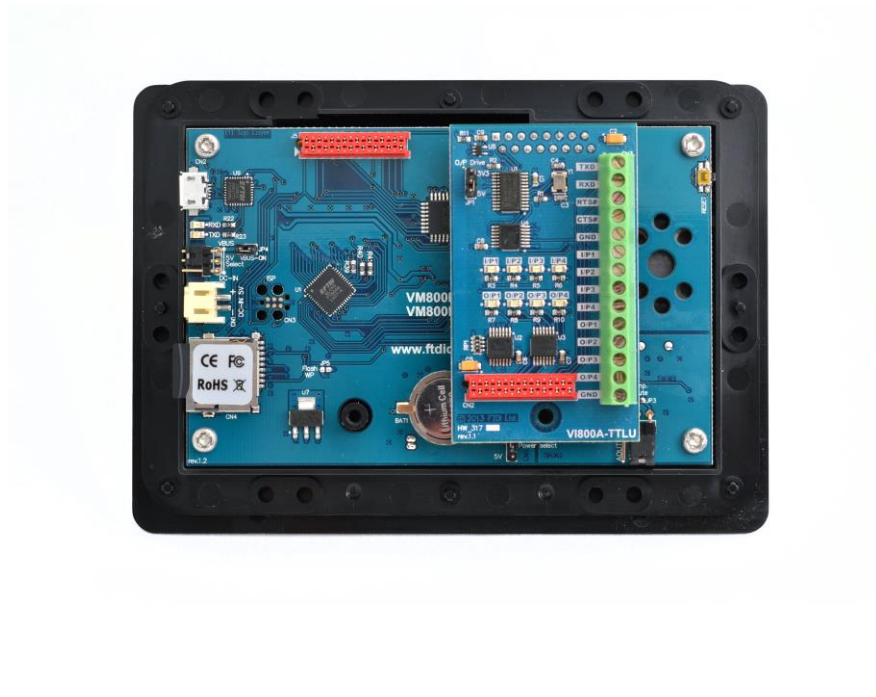
Figure 5-1 - VI800A-TTLU module connected to VM800P Plus module
