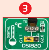
Figure 12-3: DS1820 connected to G1.7 pin
