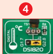
Figure 12-4: DS1820 connected to G2.0 pin
