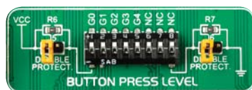
Figure 6-5: Button press level DIP switch (tri-state)
