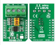
RS485 Click 3.3V is an accessory board in **mikroBus**<sup>TM</sup> form factor. The on-board **SN65HVD12** differential line transceiver is suitable for high speed bidirectional data communication on multipoint bus transmission lines. It is designed for balanced data transmission and complies with EIA RS-485 standard. This transceiver features a differential line driver and differential line receiver. Board is set to use 3.3V power supply only.
