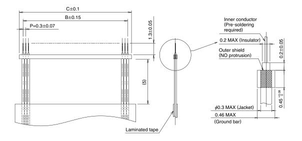
Note 1: Contact Hirose for Termination Procedures.
