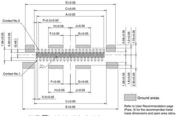
Note 1>: Area indicated must be free of conductive traces or the conductive traces must be covered by resist film.
