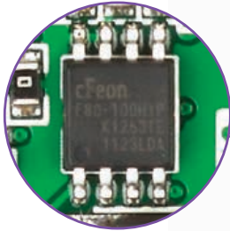
Figure 11-1: Flash memory module
