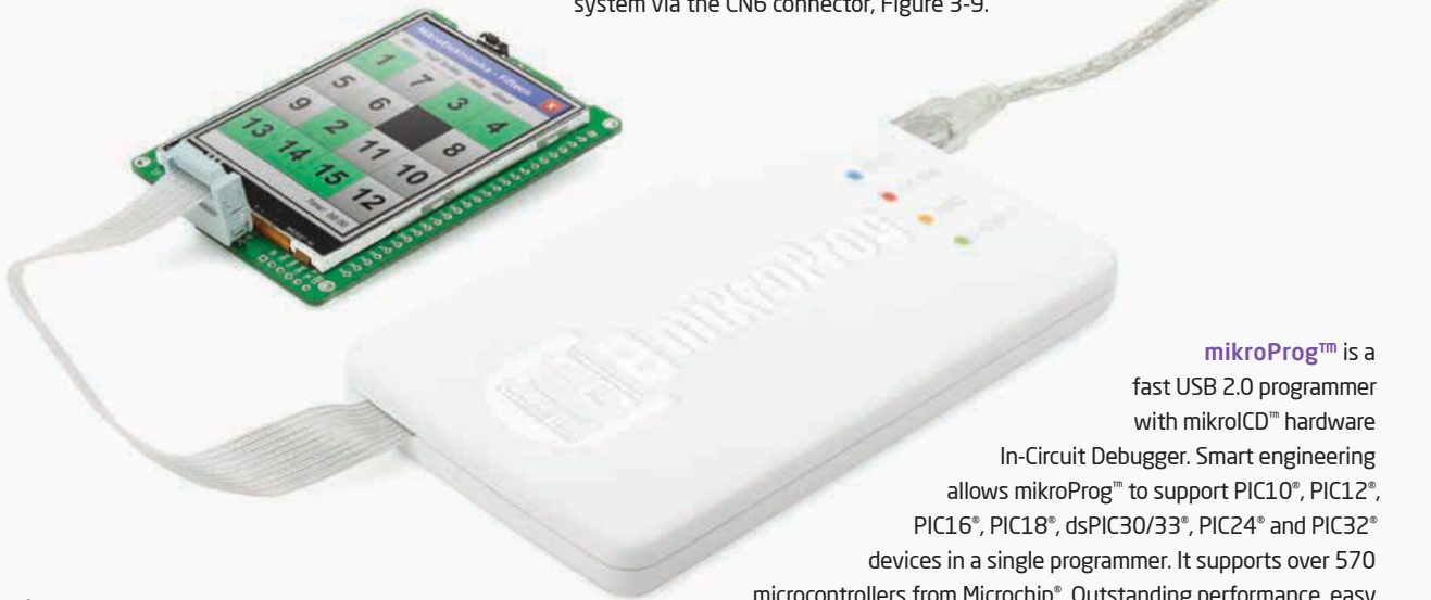
Figure 3-9: Connecting mikroProg™ to mikroMedia™
