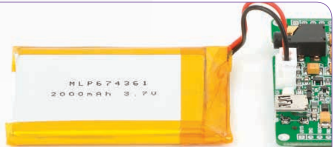
Figure 1-2: Connecting Li-Polymer battery
