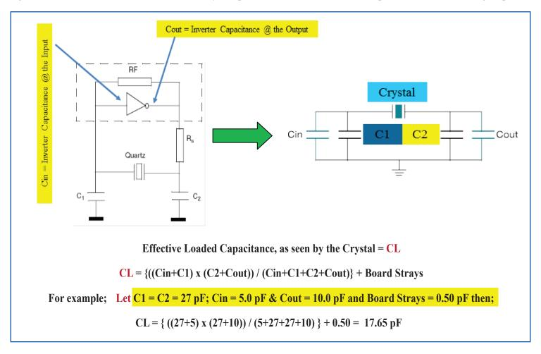
Therefore specifying a crystal with 18.0 pF plating load capacitance would be the closest match for frequency accuracy.
