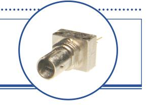
The OPF342 family fiber optic transmitters are high performance devices packaged for data communication links. This transmitter is an 850nm GaAlAs LED and is specifically designed to efficiently launch optical power into fibers ranging in size from 50/125µm up to 200/300µm diameter fiber. Multiple power ranges with upper and lower limits are offered which allows the designer to select a device best suited for the application.
