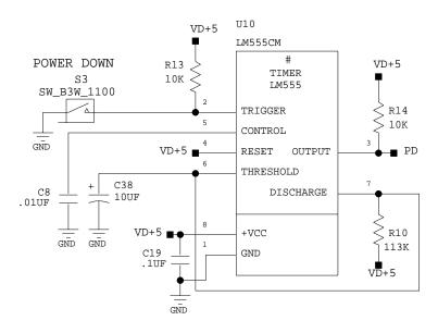
Figure 8. Power Down Circuitry
