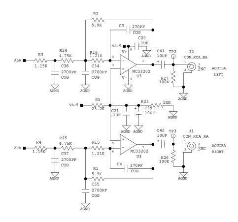
Figure 3. Analog Output Active Filter
