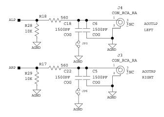
Figure 4. Analog Output Passive Filter
