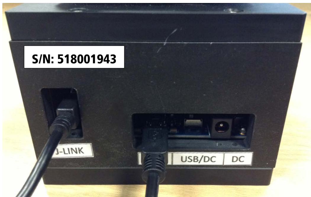
Figure 7: J-LINK cable connecting to programming jig
