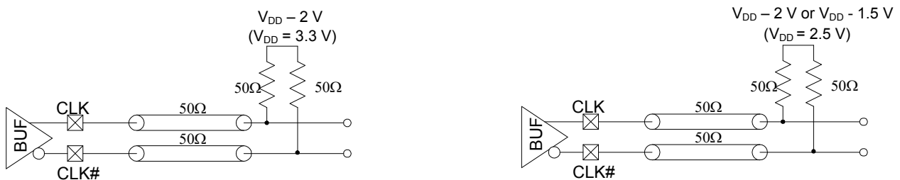
Figure 9. LVPECL Termination
