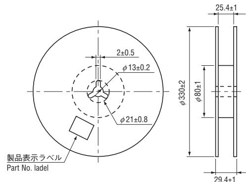
Unless otherwise specified, tolerance: ± 0.3 (Unit: mm)
