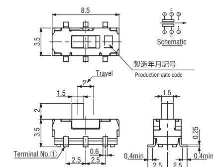
Unless otherwise specified, tolerance:  $\pm 0.3$  (Unit: mm)
