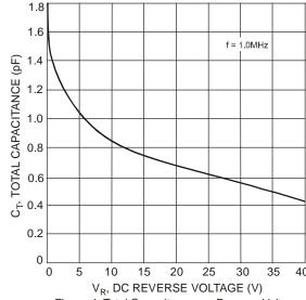
Figure 4 Total Capacitance vs. Reverse Voltage
