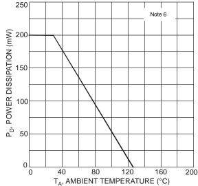
Figure 1 Power Derating Curve, Total Package
