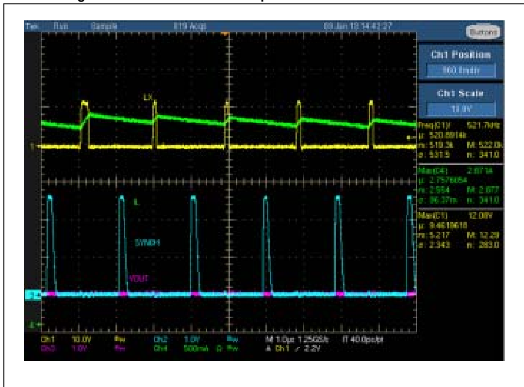
Figure 19. Peak current sense operation in overcurrent condition
