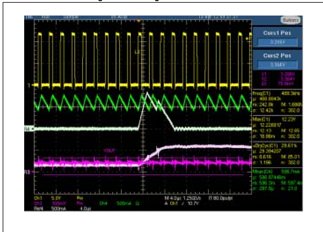
Figure 17. The regulator works in CCM
