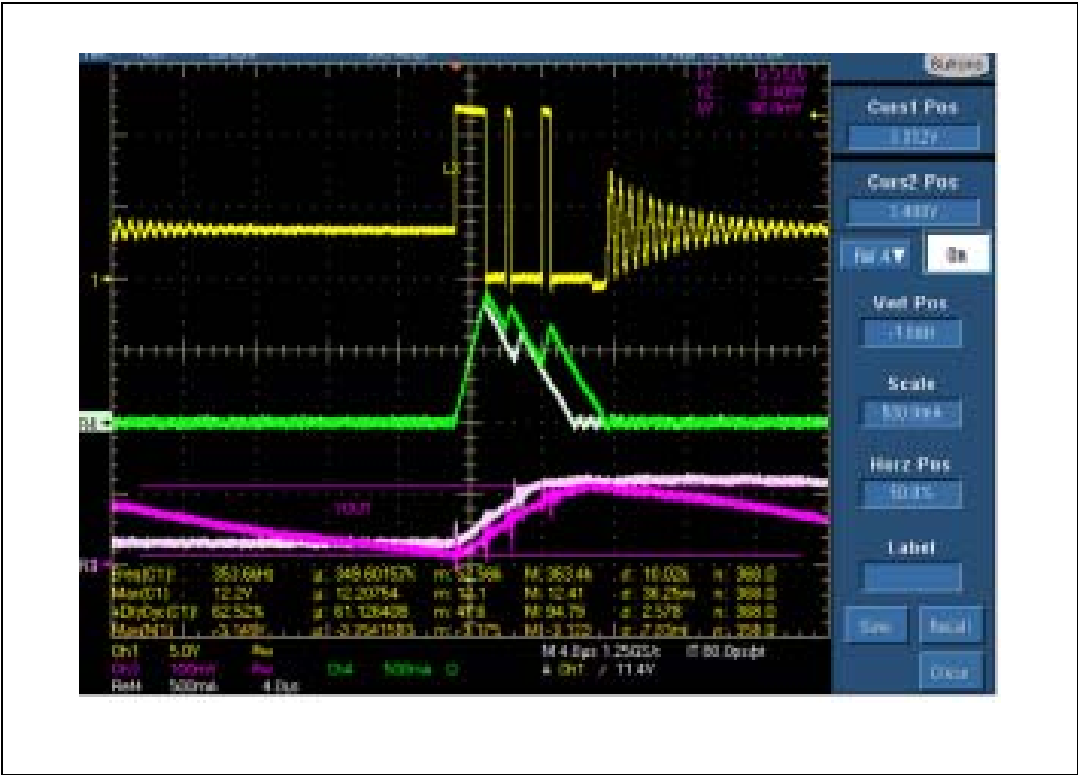
Figure 15. LCM operation over loading condition (part 1)
