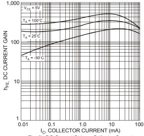
Fig. 2, DC Current Gain vs Collector Current
