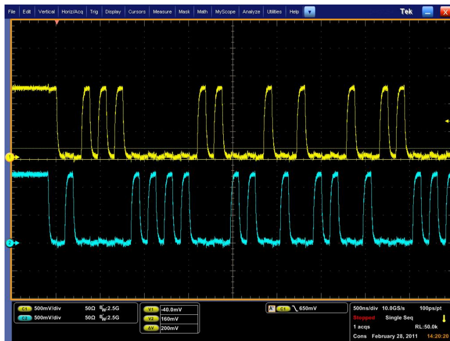
Figure 5. EMI4192 MIPI D-PHY LP Mode Measured Results
