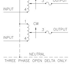
**SCHEMATIC** THREE PHASE OPEN DELTA AND SINGLE PHASE SERIES. FUSE RECOMMENDED BUT NOT SUPPLIED.
