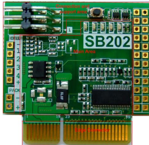
Figure 2-1. SB202 block layout.
