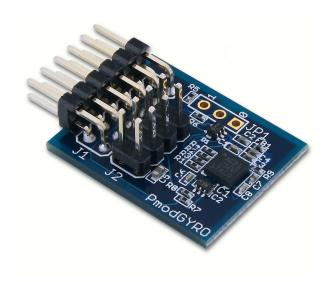
is disabled. The second interrupt, INT2, is primarily used for data ready and FIFO interrupts and maps to pin 8 on J1.
