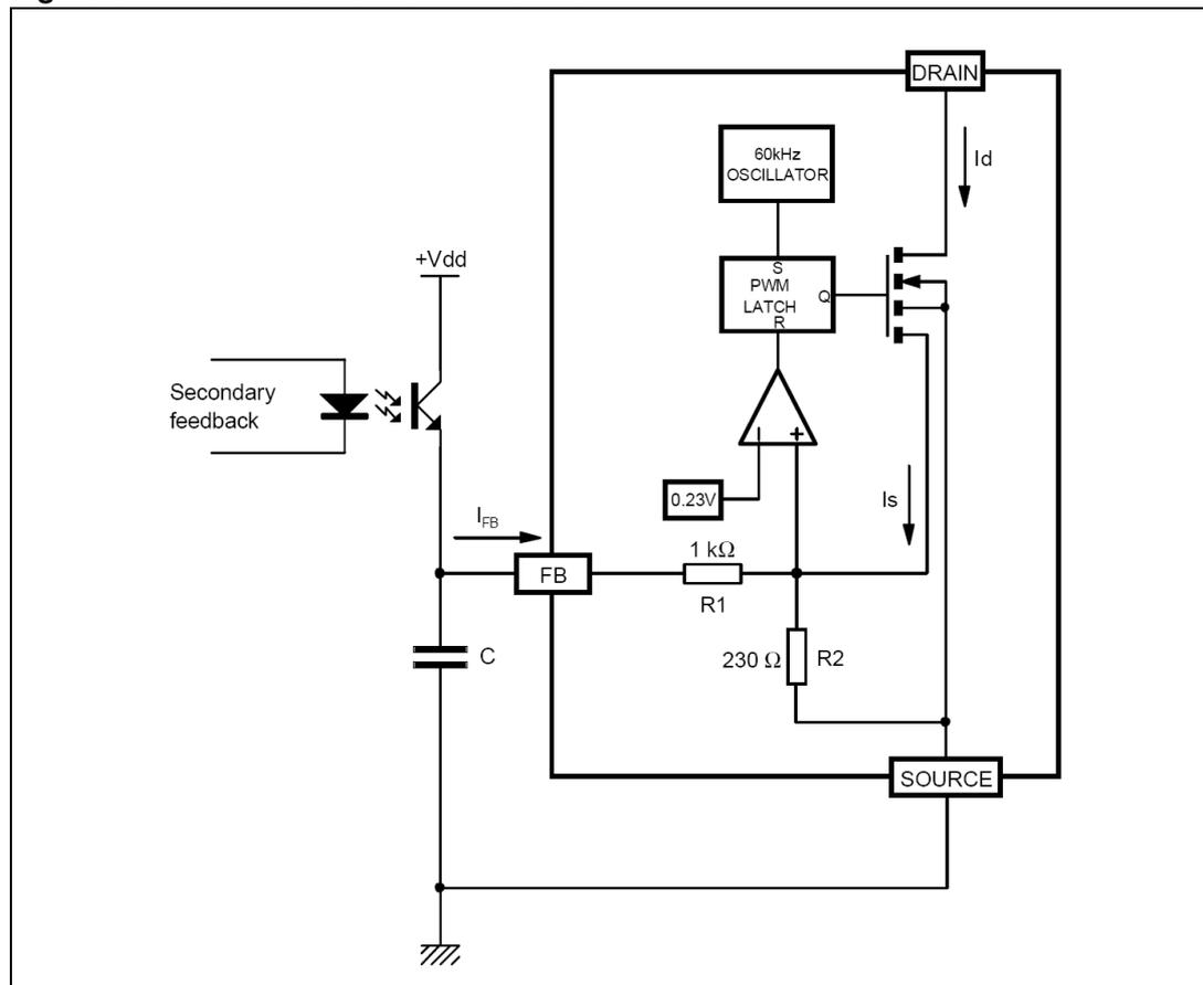
The Power MOSFET delivers a sense current  $I_S$  which is proportional to the main current  $I_D$ . R2 receives this current and the current coming from the FB pin. The voltage across R2 is then compared to a fixed reference voltage of about 0.23 V. The MOSFET is switched off when the following equation is reached:
