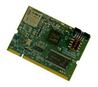
Modular RX62N based Microprocessor Plug-In System On Module
