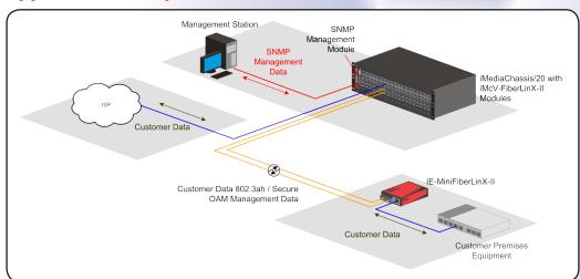
Installed here in the iMediaChassis/20, the SNMP Management Module allows for a network operator to remotely monitor and manage the functionality of all modules (iMcV-FiberLinX-II) within the chassis. Utilizing UMA, the network operator can also manage all the remote IE-Mini-FiberLinX-II devices through a single IP address assigned to the SNMP Management card.
