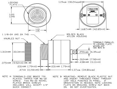
NOTE B: MOUNTING- REMOVE BLACK PLASTIC NUT AND INSERT THREADED FRONT THROUGH 125' HOLE PUNCHED IN PANEL, IF ORIENTATION IS NEEDED, NOTE LOCKING FLATS ON DRAWING. SCREW NUT BACK ON. DO NOT OVERTIGHTEN.
