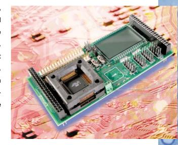
The STK502 demonstrates all the capabilitie of the Low Power ATmega169 AVR® Flash microcontroller. Two applications notes designed to run on the STK502 hardware help reduce time-to-market for designers using the ATmega169.
