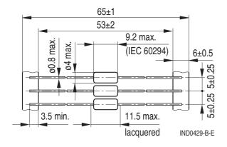
Minimum lead spacing 12.5 mm
