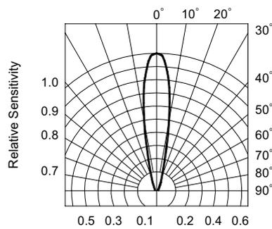
FIG.5 SENSITIVITY DIAGRAM
