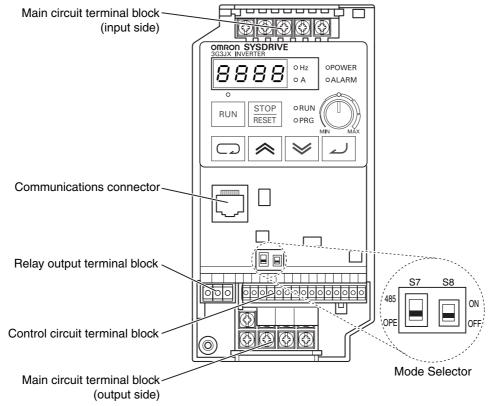
Note: This illustration shows the terminal block with the front cover removed.
