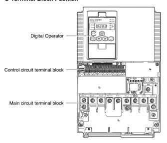
Note: This illustration shows the terminal block with the Terminal block front cover removed.
