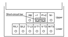
Terminal Arrangement 3G3MX-A2015 to A2037 3G3MX-A4004 to A4037 3G3MX-AE007 to AE022
