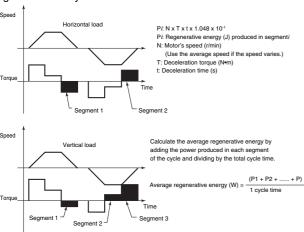
**Note 1.** The speed is positive when the motor is rotating forward and the torque is positive when it is in the forward direction.
