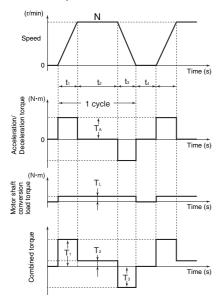
Use the Servomotor's Motor Selection Software to calculate the motor conversion inertia, effective torque, and maximum torque shown above.
