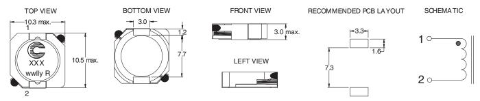
Dimensions are in millimeters.
