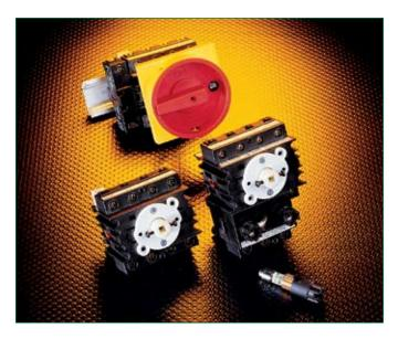
The LFFS series fusible switches eliminate the need for a separate fuse block by integrating a three pole fuse holder into the switch body. This saves precious panel space and reduces wiring time. These rodoperated devices are UL Listed and CSA Certified.
