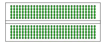
The BB300 breadboard tie-points are connected in 60 vertical columns (the green lines) with 5 connected holes in each. This is the circuit area. When an integrated circuit is plugged into the breadboard, each I.C. pin has a column. There are no horizontal running connections on the BB300.
