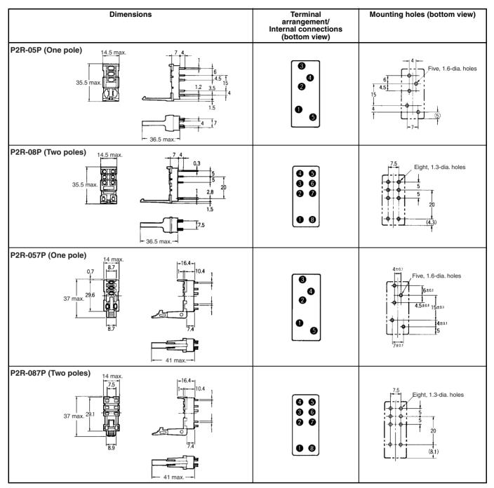
Note: When indicator modules with an I/O SSR are used, the No. 1 pin becomes positive.
