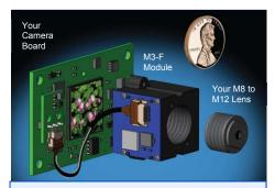
Flexibility and Precision: M3-F modules are easily integrated with your camera board and lens. The M3-F is a complete, drop-in focus solution that requires no more space than a fixed lens holder.
