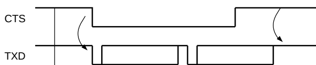
Figure 36-29. Transmitter Behavior when Operating with Hardware Handshaking
