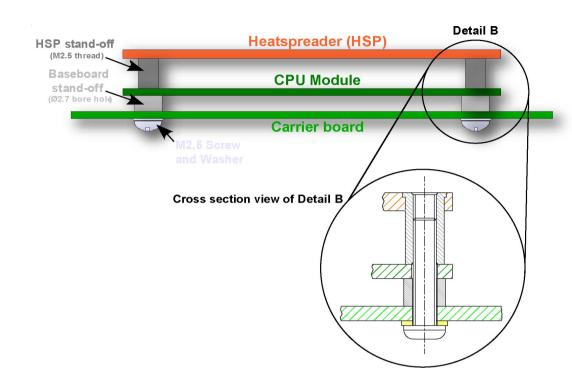
Picture 3: Complete assembly using threaded heatspreader
