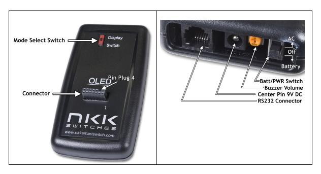
The **Mode Select Switch** has two settings; "Switch" is for the OLED (64x48) switches and "Display" is for the OLED (52x36) displays.
