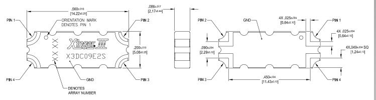
Dimensions are in Inches [Millimeters] X3DC09E2S Mechanical Outline
