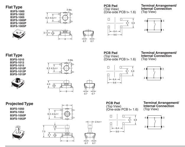
**Note:** Unless otherwise specified, a tolerance of  $\pm 0.4$  mm applies to all dimensions. No terminal numbers are indicated on the Switches.
