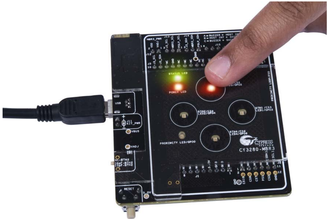
Figure 5-15. Auto-Reset Feature - LED Output on Button Touch
