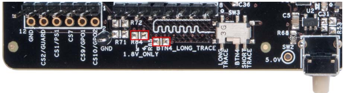
Figure 4-6. R84 and R85 for Externally Regulated Operation at 1.8 V
