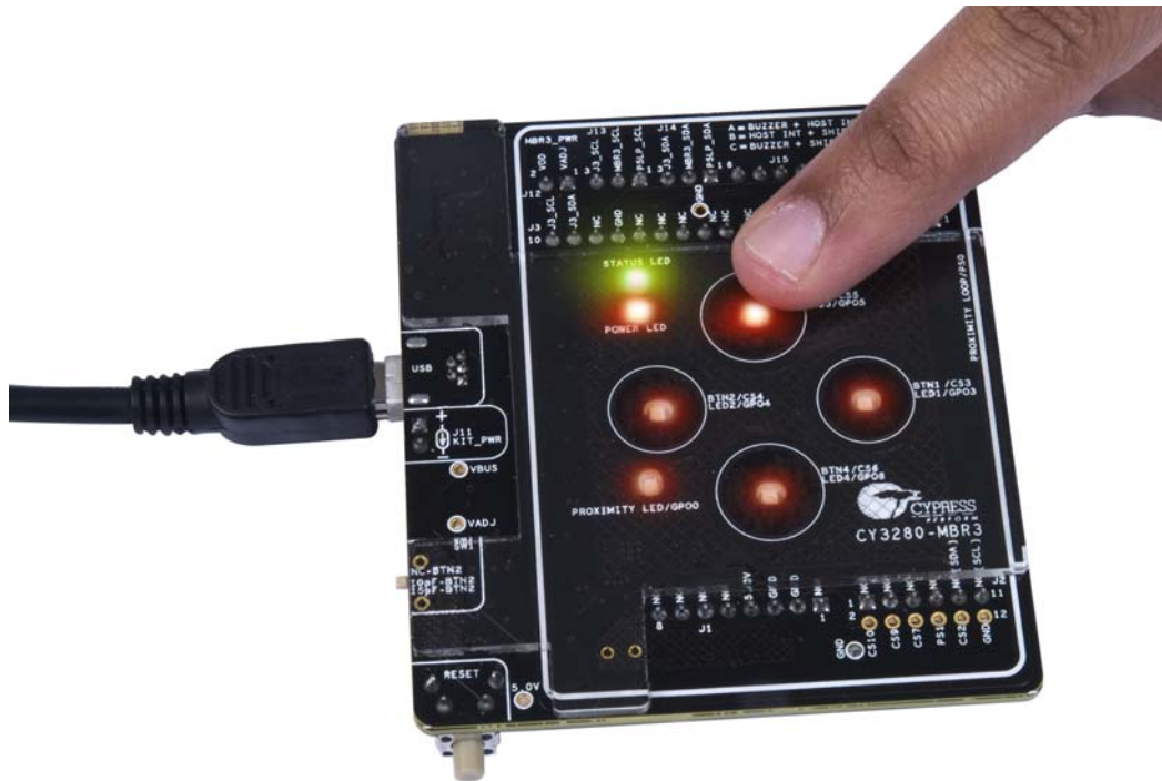
Figure 5-8. LEDs with 93 Percent Brightness on Button Touch
