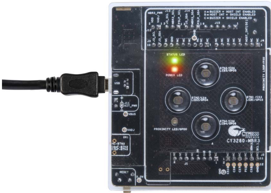
Figure 5-17. Verify Water Tolerance - Without Finger
