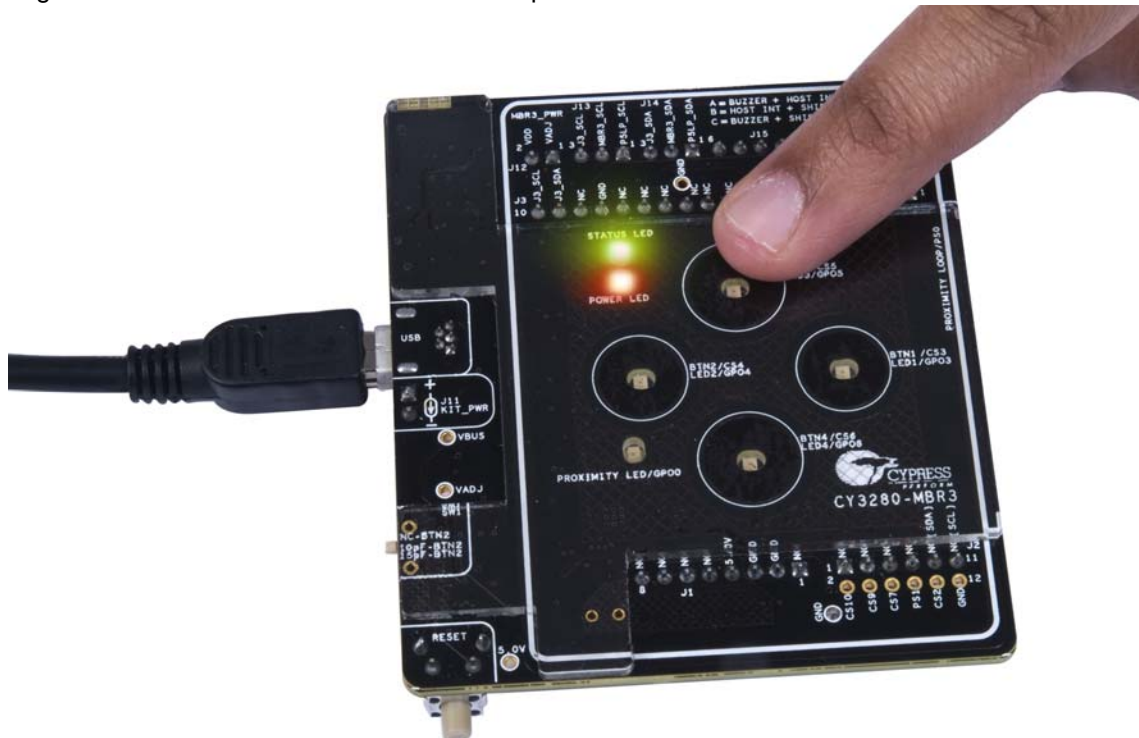
Figure 5-16. Auto-Reset Feature - LED Output Five Seconds After Button Touch
