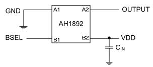
Note: CIN is for power stabilization and to strengthen the noise immunity, the recommended capacitance is 100nF typical
