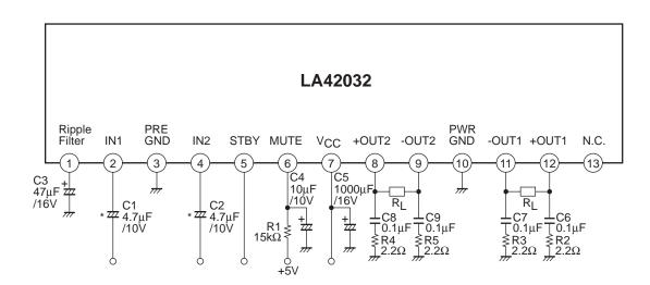
\* LA42032 employs the zero-bias type input circuit, with the input pin potential being nearly zero (about 0.01V). Accordingly, the polarity must be determined according to the DC potential of a circuit connected to the previous stage of LA42032.
