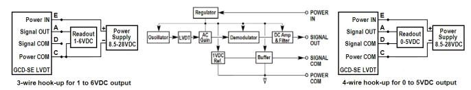
A through E: Connector pin assignments
