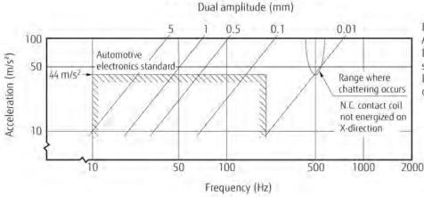
Frequency: 10~2000 Hz Acceleration: 100 m/s2 max. Direction of vibration: see diagram below Detection level: chatter > 100 µs
