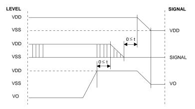
Please maintain the above sequence when turning on and off the power supply of the module. If  $V_{\text{EE}}$  is supplied to the module while internal alternate signal for LCD driving (M) is unstable or RESET is active, DC component will be supplied to the LCD panel. This may cause damage to the LCD module.
