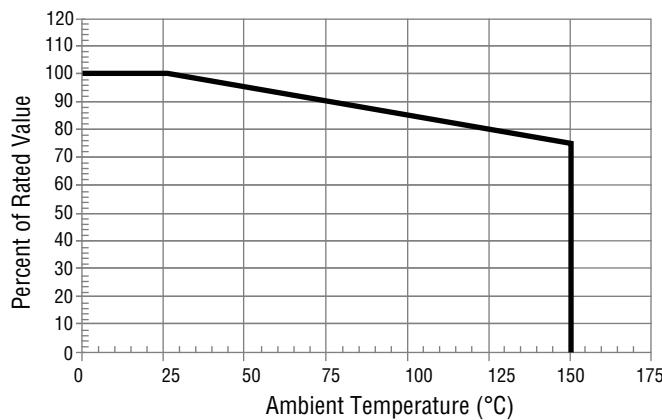
*This graph shows the typical device surge current derating versus ambient temperature when subjected to the 8/20  $\mu$ s current waveform per the IEC 61000-4-5 specification.*
